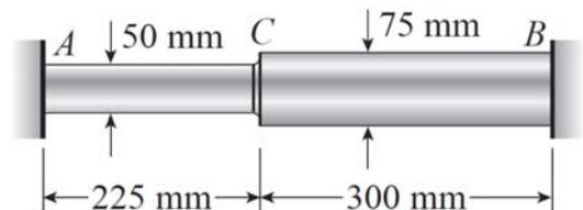
(a) Calculate the following quantities: (1) the compressive force  $N$  in the bar; (2) the maximum compressive stress  $\sigma_c$ ; and (3) the displacement  $\delta_C$  of point C.
